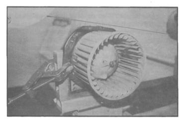
10. The last slide is a small blower fan from an automobile.
