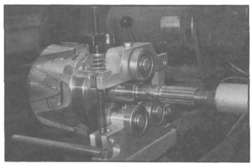
9. Oil drive alternator, balance time is 20 minutes, rate is 2 times the shop rate, balance on 1 column.
