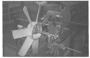
Number three is an air duct fan with a balance time of 40 minutes.
