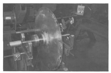
Our first slide is of a shaping disc, approximately 2<sup>1</sup>/<sub>2</sub> feet in diameter. It is used in the wood products industry. The time taken to complete the job is 35 minutes.
