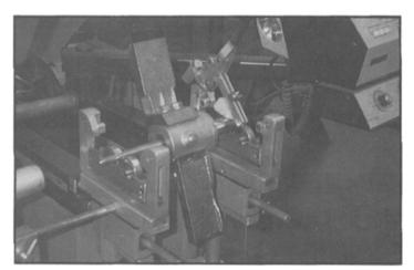
4. Next we have an impeller that throws steel shot. The steel shot or balls wear away the front or leading side of the impeller. Rather than throw it away, the fix is to turn the impeller 180 degrees on the hub. But guess what, it then needs balancing. Total balancing time is 15 minutes per unit.
