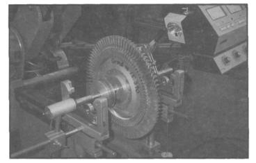
8. This is a compressor wheel followed by a compressor section from the same engine. These are Vietnam era helicopter engines, now used in other applications, specifically hydroplane racing.
