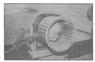
The last slide is a small blower fan from an automobile.
