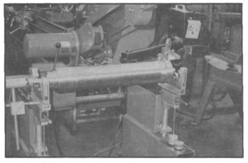
Our fifth slide is of a centrifuge bowl. This is used as an oil separator in a marine application. Balance time is approximately 45 minutes.
