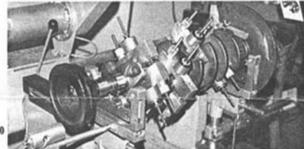
8. A belt sander is recommended for removing weight from rod
