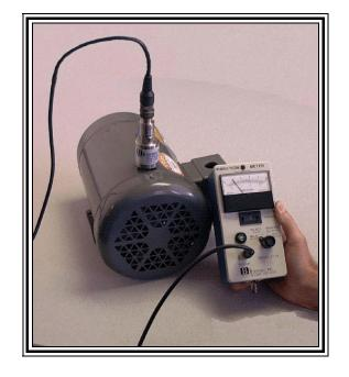
INPUT: CONTROLS: Accelerometer (100 mV/g)
